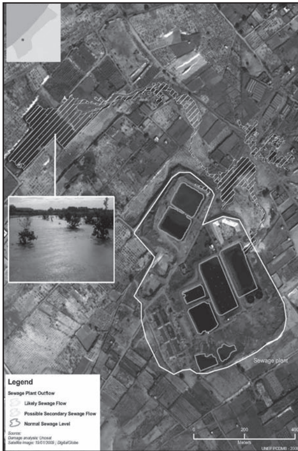
Figure 13: Extent of sewage flood from Al Zaitoun sewage treatment plant as a result of Operation of Cast Lead (Image from 19th January 2009). 188
